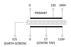
NOTE: 220/240V PRIMARY VOLTAGE AND 110V SECONDARY VOLTAGE RANGES ARE SHOWN FOR GUIDANCE PURPOSES ONLY, CONNECTION INFORMATION IS ALSO VALID FOR OTHER PRIMARY VOLTAGE AND SECONDARY VOLTAGE COMBINATIONS.
